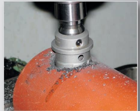
Bohren in Rohre
