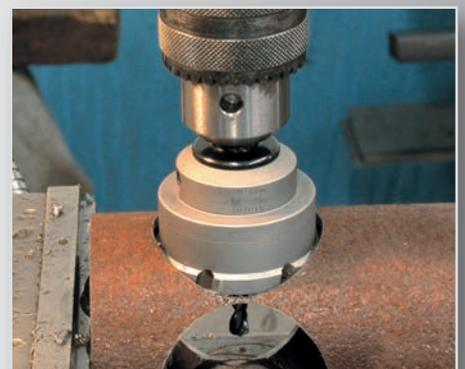
Bohren in Rohre
