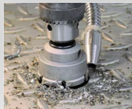
Drilling in checker sheet
