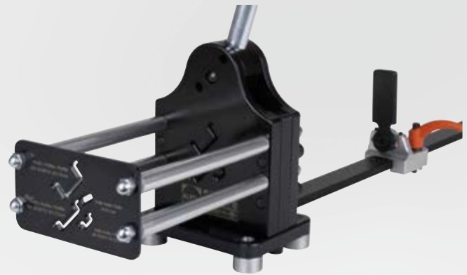
Guidance fixture for 90° angle-precise cutting
