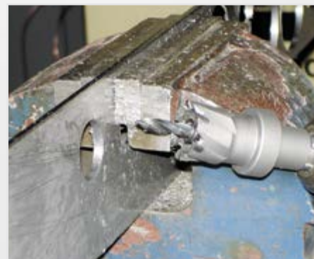
Free-hand drilling up to Ø 30 mm
