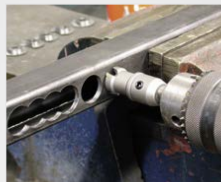
Drilling in square profiles
