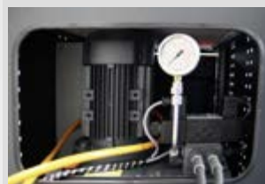
Dual-circuit hydraulic unit in cabinet base
