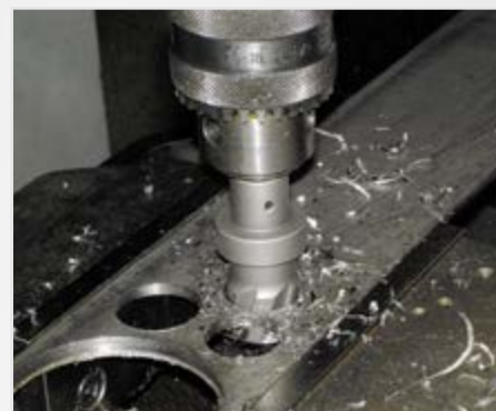
Drilling flat steels
